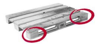
A single upper or lower leading board is damaged so that more than one nail or screw shank is revealed.
