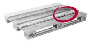
More than two upper or lower leading boards are damaged and reveal one nail or screw shank for each board.
